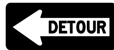
M4-10L BLACK ON WHITE 48" X 18" INSTALLED ON TYPE III BARRICADE
